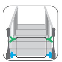
Determine location where you need Y-Spindles and insert the Y-Spindle(s) in those locations.
