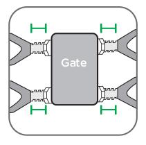
Using the wrench provided with the gate, and while following the instructions for proper installation of the gate, tighten the four spindles securely.
