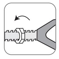
Hand tighten the nuts on all spindles until they are extended equally and touch the banisters/spindles or wall.
