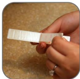
Thoroughly clean the surface the adhesive will be attached to. Make sure the surface is dry. Remove the adhesive protective liner.
